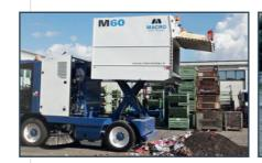
Very large volumes of dry collected waste. 6 m³ hopper and 6000 kg payload is the highest capacity on the market, allowing long
