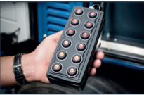
Easy-to-use keypads to operate the machine. "EasyStart" single button for all required functions on/off (CB).
